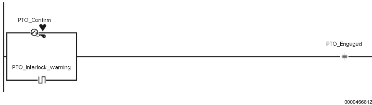
Figure 173 Logic for PTO Gauge Cluster Lamp
