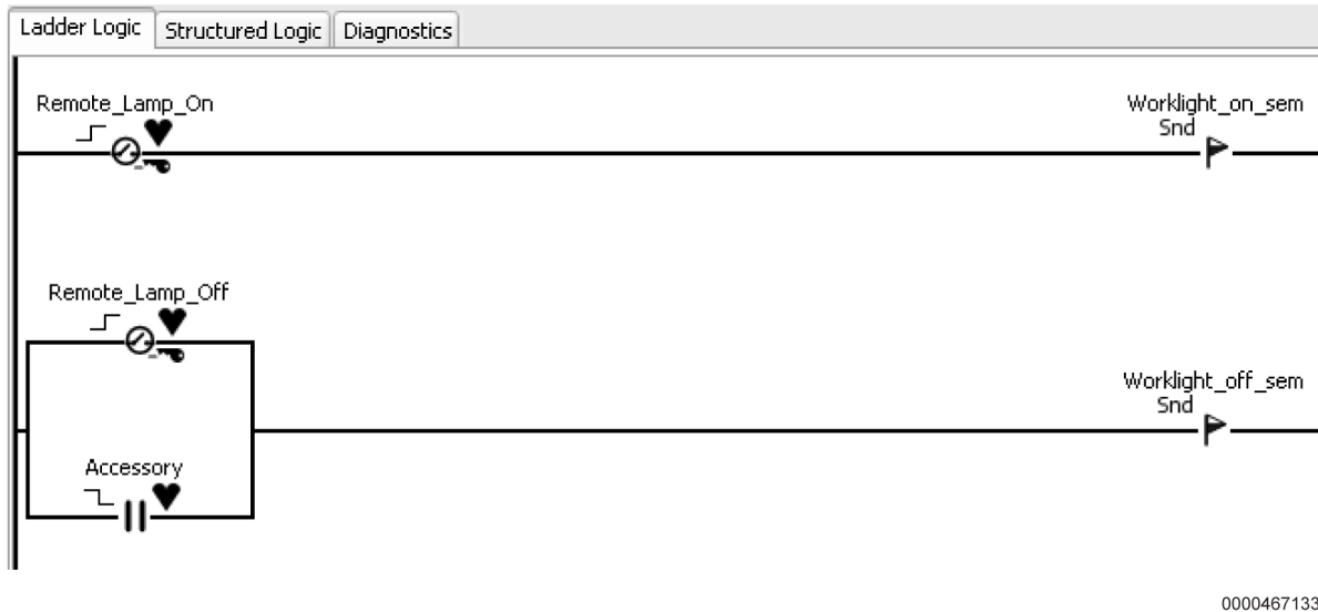
Figure 82 Example of Controlling the Work Light Channel Post 2007 Vehicles
