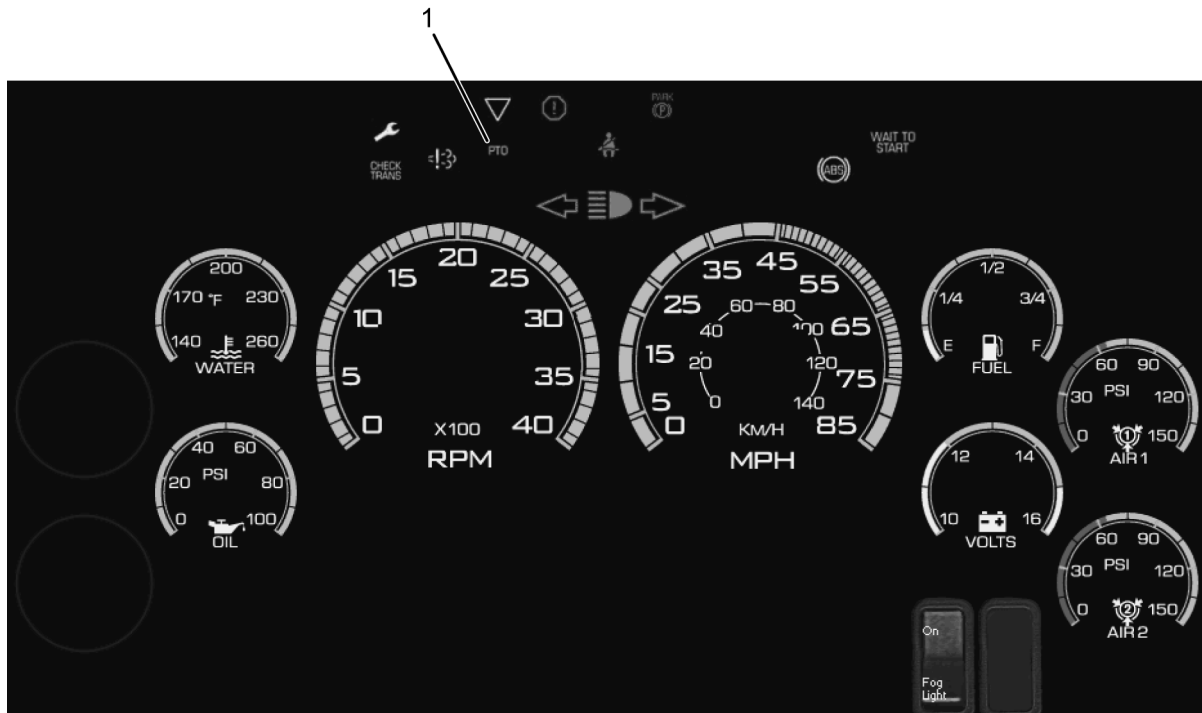
Figure 89 Key Off Functionality in the Gauge Cluster (Post 2007)
