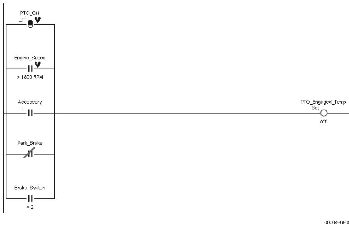
Figure 166 Set the Variable OFF when One or More Interlocks Are Not Met
