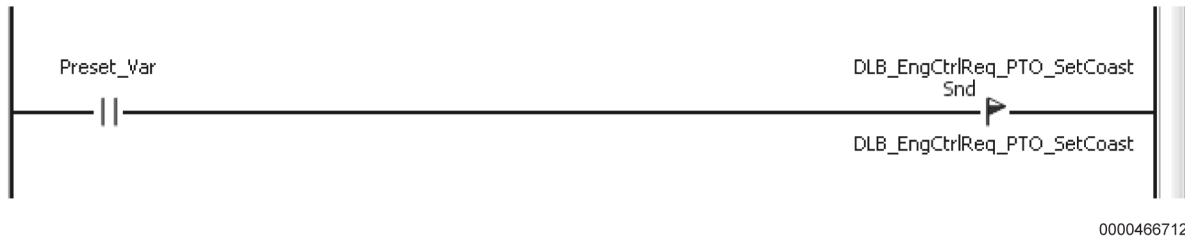
Figure 127 A26 Preset Engine Speed Control
