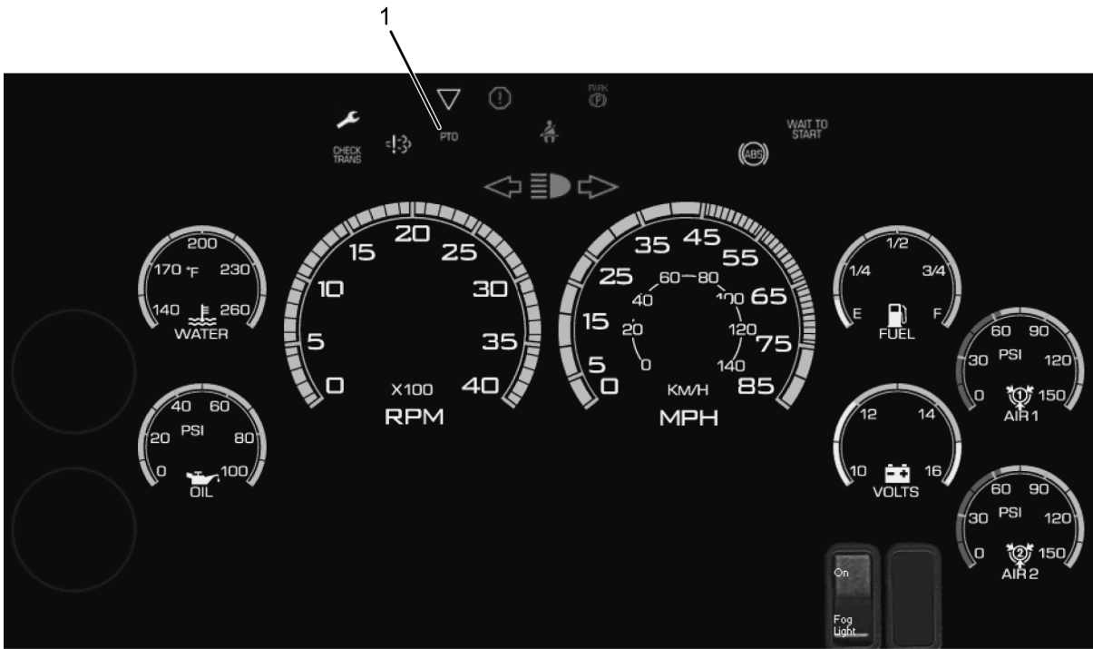
Figure 175 Gauge Cluster View with PTO Light (Built 2007 or Later)
