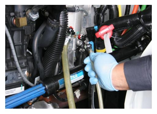
2. Disconnect 15-637-01-8 Return Adapter (fuel return) from the fuel return on the fuel filter housing assembly.
