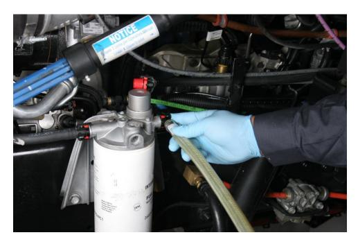
5. Disconnect 15-637-01-4 Supply Adapter (fuel inlet) from fuel supply on fuel filter.
