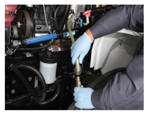
4. Connect 15-637-01-2 Supply Line (fuel supply) from the 15-637-01-1 Clean Fuel Source Tank to 15-637-01-4 Supply Adapter (fuel inlet) quick coupler.
