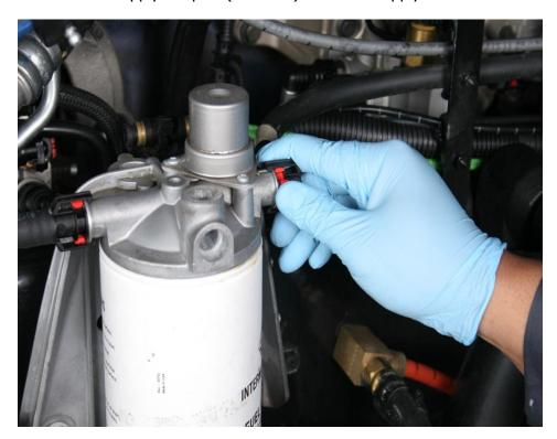
6. Remove disposable clean air/fuel caps from openings and connect fuel supply line to fuel supply on fuel filter housing.
