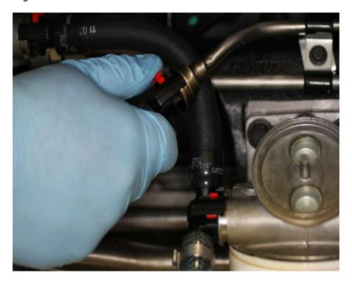
3. Remove disposable clean air/fuel caps from openings and reconnect the fuel return line to the primary fuel filter assembly.
