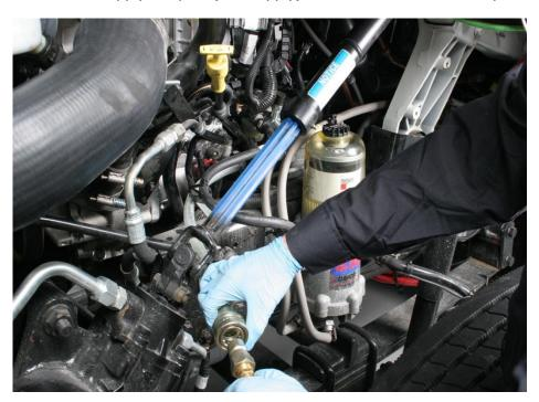
5. Install 15-637-01-2 Supply Line (fuel supply) from 15-637-01-1 Clean Fuel Source Tank to 15-637-01-4 Supply Adapter (fuel inlet) quick coupler.
