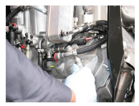
10. Install 15-637-01-7 Return Adapter (fuel return) to fuel return connector on fuel cooler assembly.
