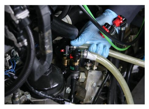
9. Install 15-637-01-5 Return Adapter (fuel return) to fuel return line brass fitting.
