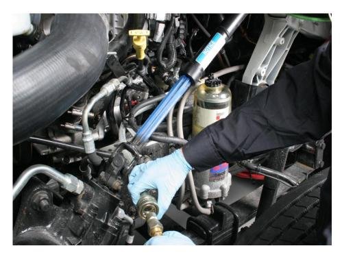
4. Disconnect (fuel supply) line for the 15-637-01-1 Clean Fuel Source Tank at 15-637-01-4 Supply Adapter (fuel inlet) quick coupler.
