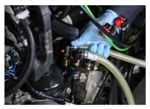
2. Disconnect 15-637-01-5 Return Adapter (fuel return) from the brass fitting (fuel return).
