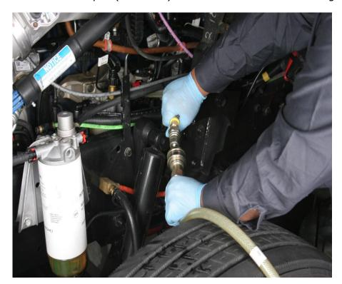
9. Install 15-637-01-3 Return Line (fuel return) on 15-637-01-1 Clean Fuel Source Tank to 15-637-01-5 Return Adapter (fuel return) quick coupler.
