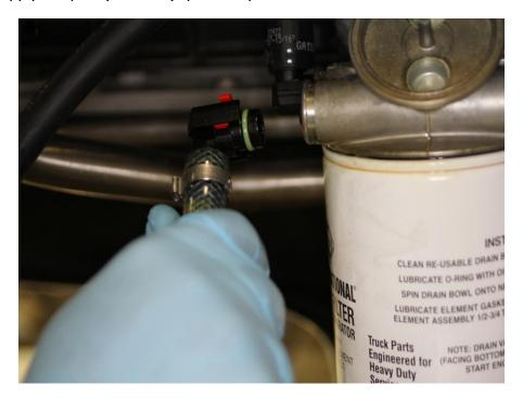
5. Disconnect 15-637-01-4 Supply Adapter (fuel inlet) from fuel supply on primary fuel filter assembly fitting.
