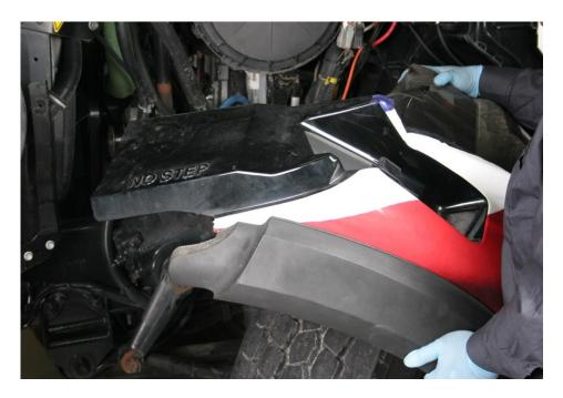
2. Remove left side fender bolts and remove fender, and place out of the way.
