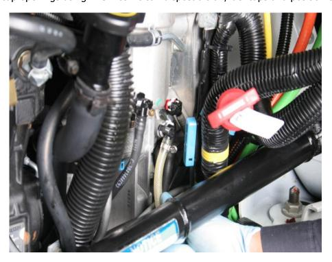
5. Connect 15-637-01-4 Supply Adapter (fuel inlet) to the fuel supply connector on the fuel filter housing assembly.
