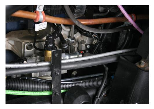
3. Remove disposable clean air/fuel caps from openings and connect fuel return line to fuel return on fuel filter housing.
