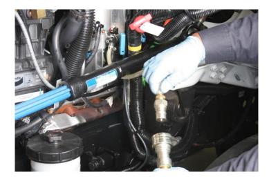
6. Connect 15-637-01-2 Supply Line (fuel supply) from the 15-637-01-1 Clean Fuel Source Tank to 15-637-01-4 Supply Adapter (fuel inlet) quick coupler.
