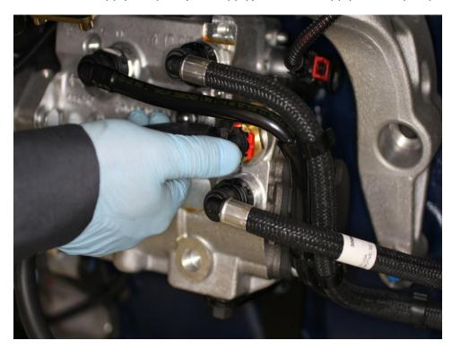
6. Remove disposable clean air/fuel caps from openings and reconnect the fuel supply line to the fuel supply on the fuel pump.
