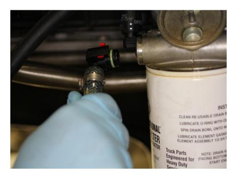
3. Connect 15-637-01-4 Supply Adapter (fuel inlet) to the fuel supply fitting on the primary fuel filter assembly.
