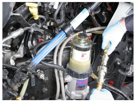
1. Disconnect 15-637-01-3 Return Line (fuel return) for the 15-637-01-1 Clean Fuel Source Tank 15-637-01-5 Return Adapter (fuel return) Line Adapter quick coupler.
