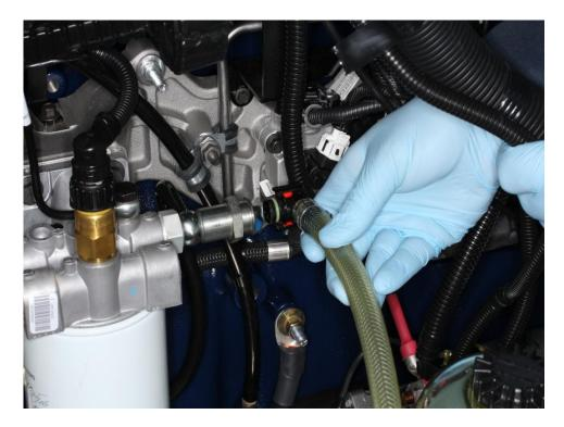
2. Disconnect 15-637-01-5 Return Adapter (fuel return) from fuel return on fuel filter.
