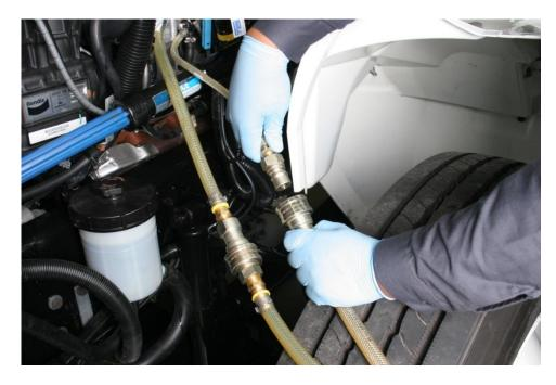
1. Disconnect 15-637-01-3 Return Line (fuel return) for the 15-637-01-1 Clean Fuel Source Tank at 15-637-01-8 (fuel return) Line Adapter quick coupler.
