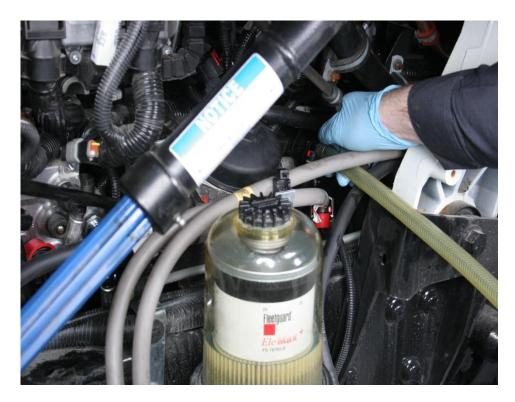
2. Disconnect 15-637-01-5 Return Adapter (fuel return) from the engine fuel return connection.
