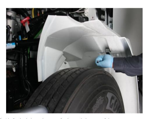
2. Remove left side fender bolts and remove fender, and place out of the way.
