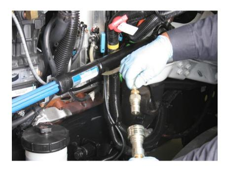
4. Disconnect 15-637-01-2 Supply Line (fuel supply) for the 15-637-01-1 Clean Fuel Source Tank at 15-637-01-4 Supply Adapter (fuel inlet) quick coupler.
