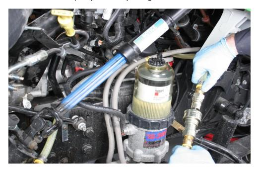
9. Install 15-637-01-3 Return Line (fuel return) on 15-637-01-1 Clean Fuel Source Tank to 15-637-01-5 Return Adapter (fuel return) quick coupler.
