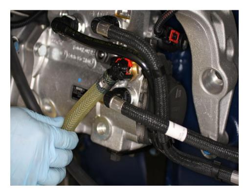
5. Disconnect 15-637-01-6 Supply Adapter (fuel supply) from fuel supply on fuel pump.
