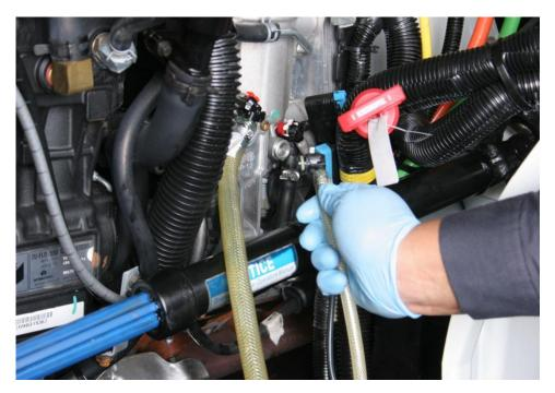
7. Connect the 15-637-01-8 Return Adapter (fuel return) to the fuel return connector on the fuel filter housing assembly.
