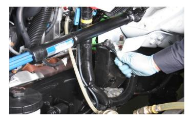
7. Remove air compressor discharge line bracket bolts and position bracket out of the way.
