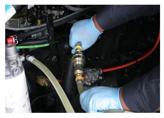
1. Disconnect 15-637-01-3 Return Line (fuel return) for the 15-637-01-1 Clean Fuel Source Tank 15-637-01-5 Return Adapter (fuel return) quick coupler.
