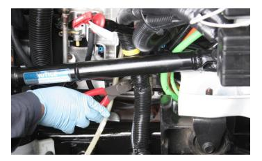
8. Cut two wire ties for the chassis harness and air lines that are near the left side body mount and position out of the way.
