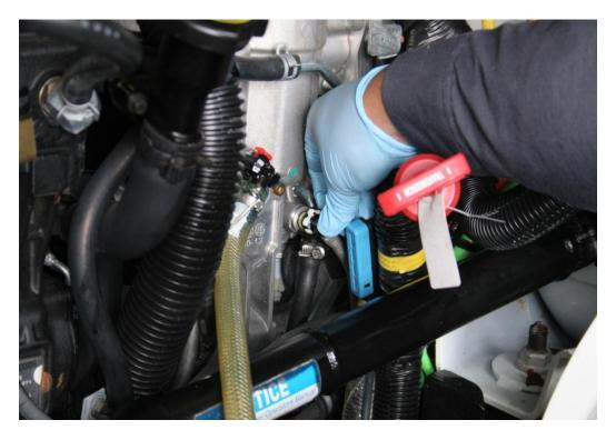
3. Remove disposable clean air/fuel caps from openings and reconnect the return line to the fuel filter housing assembly.
