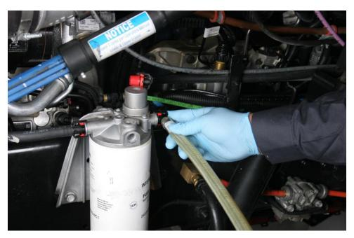
4. Install 15-637-01-4 Supply Adapter (fuel inlet) to fuel supply on fuel filter.
