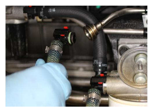
2. Disconnect 15-637-01-8 Return Adapter (fuel return) from the fuel return on the primary fuel filter assembly fitting.
