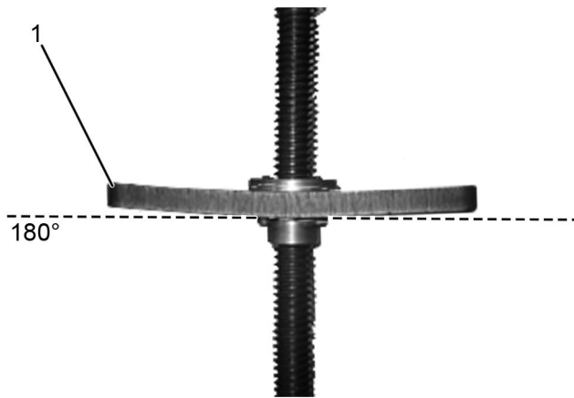
Figure 1. Damaged Puller Plate.
