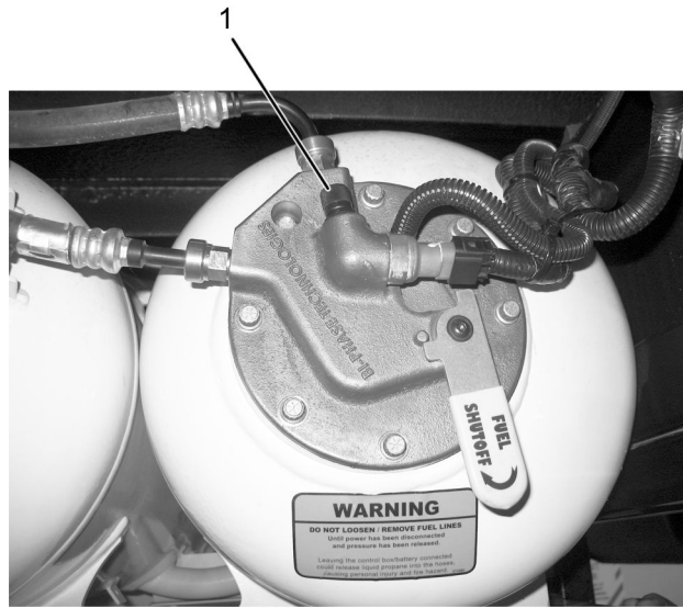
Figure 2. Fuel Shutoff Valve.
