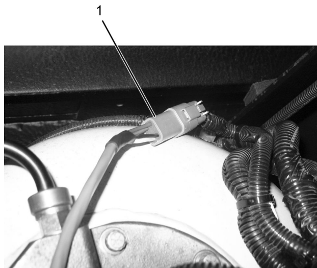
Figure 3. 15-127-01 3-Switch Box – LPDM Harness Connection.
