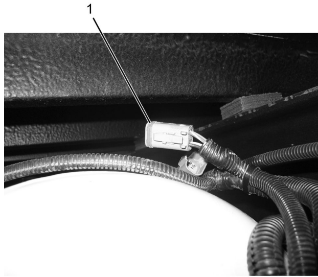
Figure 2. Liquid Propane Distribution Module (LPDM) Harness.
