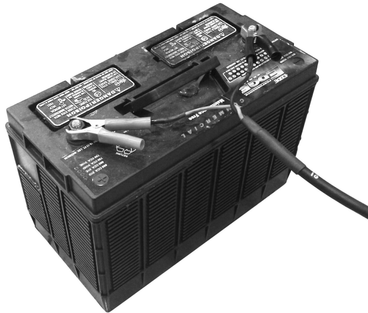
Figure 4. 15-127-01 3-Switch Box – Battery Connection.
