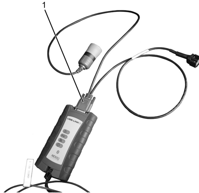
Figure 2. 08-801-01 Electric Vehicle Adapter Cable Pre-Assembly
