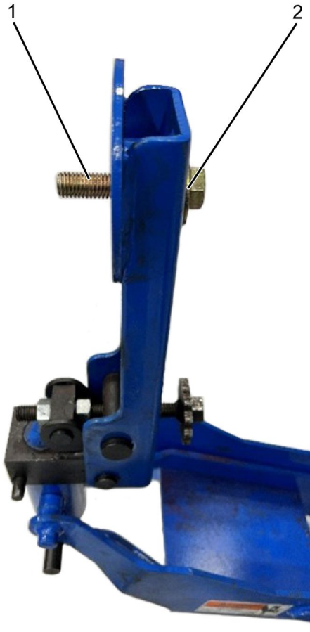
Figure 3. Clutch Kit Assembly
