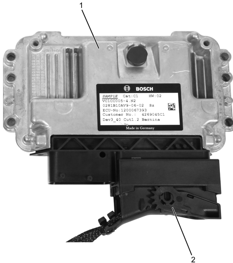
Figure 4. Programming harness 12-801-01-19 connected to PIM
