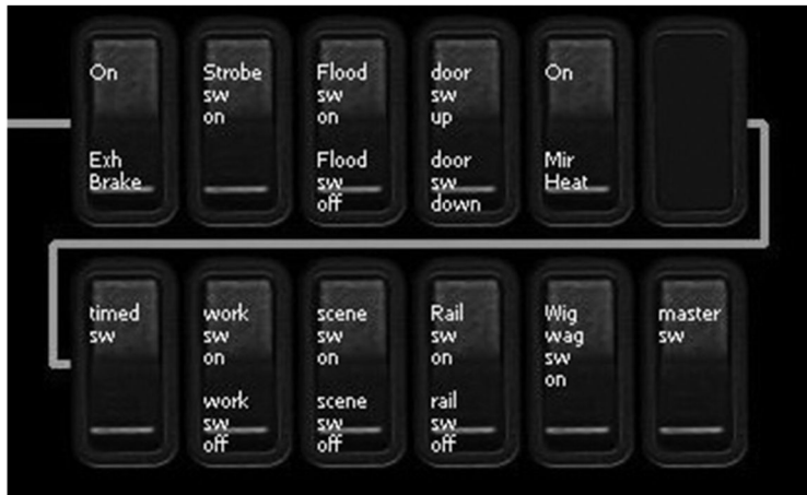
Figure 124 Master Switch Moved to Lower Bank
