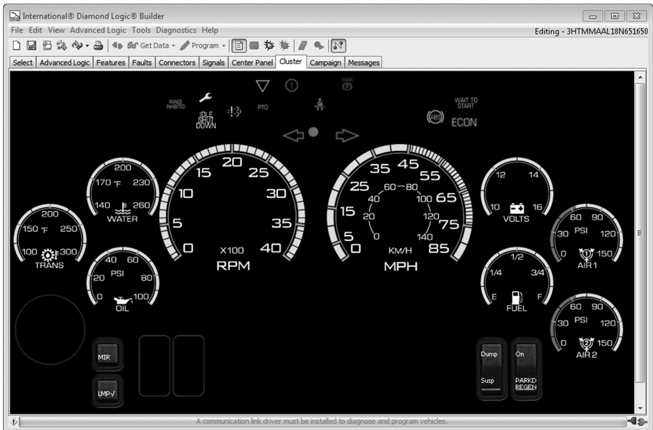
Figure 125 Cluster Tab with Two Vacant Switch Locations (Lower-Left)
