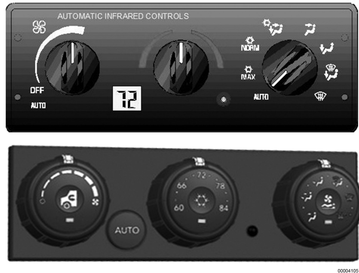
Figure 11 Two Examples of HVAC Control Panels
